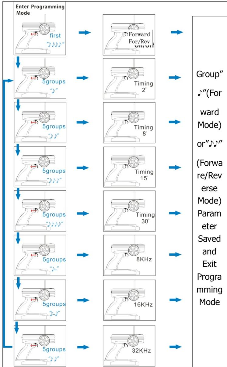
This series ESC can be set some simple function values via the transmitter, but the more function value setting have to use prog-box or PC via USB link wire.
